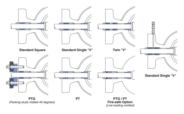
**Figure 3: Typical Packing Configurations**
