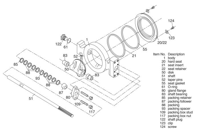
Figure 5: Exploded Body Sub-Assembly
