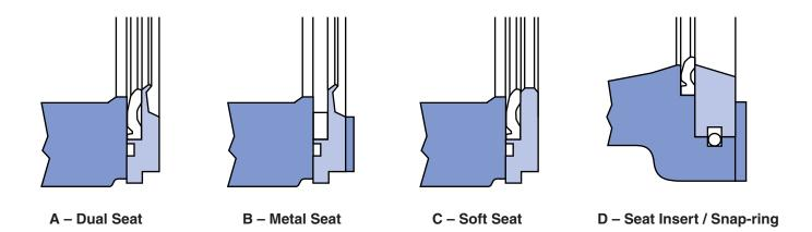
**Figure 1: Seat Retainer Configurations**
