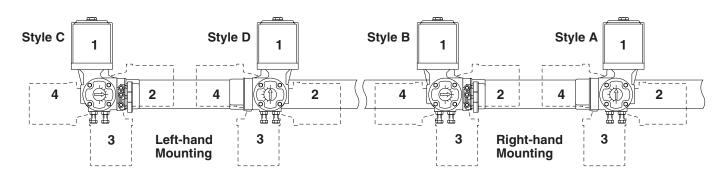
**Figure 4: Transfer Case Mounting**
